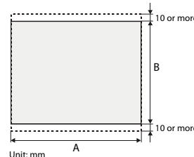
A space of at least 10 mm at the upper and lower side of the GOT is required to allow for the attachment of mounting fixtures.
