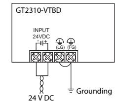
Use the thickest cable possible (max. 2 mm<sup>2</sup>) to minimize the voltage drop and start twisting them close to the connection terminals. Tighten the terminal screws securely with a torque of 0.5 to 0.8 Nm. Use commercially available terminal ends for M3 screws for connection of the power supply (see figure below).
