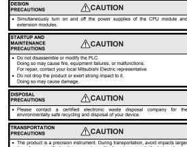
than those specified in the general specifications by using dedicated packaging boxes and shock-absorbing palettes. Failure to do so may cause failures in the product. After transportation, verify operation of the product and check for damage of the mounting part, etc.
