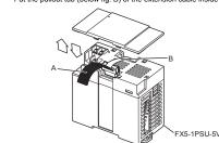
3) Push out DIN rail mounting hook. 4) Fit the upper edge of the DIN rail mounting groove (below fig. C) onto the
