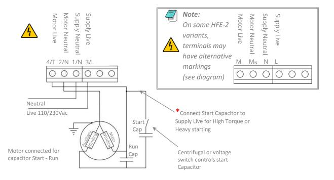
Extra starting torque may be needed for loads which have a particularly 'sticky' starting characteristic. This can be achieved by rearranging the internal connection of the starting capacitor, bringing the connection out and connecting to the supply side of the starter as shown.
