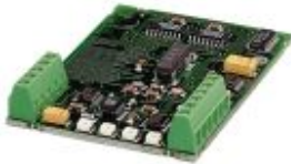
Universal I/O module in the form of a daughterboard
