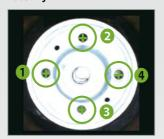
This inspection item counts how many labels there are of the specified colour and size and measures the area or center position of the specified label.
