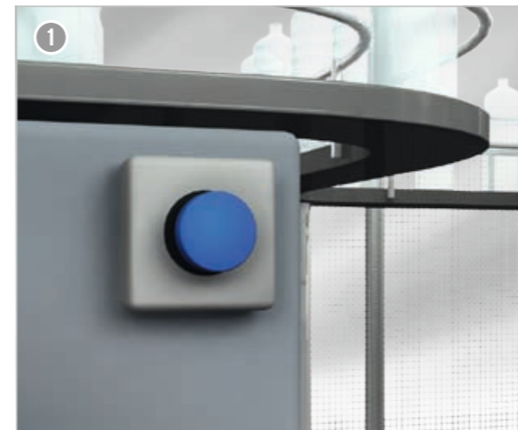
Local pre-reset pushbutton inside the machine that needs to be pressed before the safety system can be reset
