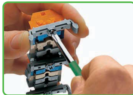
Terminal strip with fixing flanges, screw mounting of 209-123 mounting adapter (The distance between mounting adapters should be 35 - 40 mm / 1.378 - 1.575 in max.).
