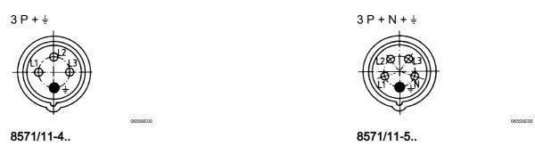
Arrangement of the socket contacts and terminal markings in the 6h position (view from the front side of the shrouded socket outlet to the socket contacts)
