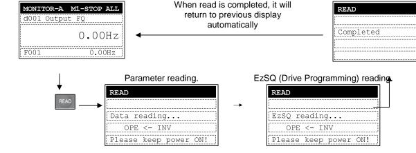
**NOTE:** All inverter parameters saved in LCD digital operator are overwritten after the key is pressed.
