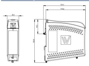
**Dimension W x H x D**  $34 \times 123 \times 121 \text{ mm} (1.33 \times 4.84 \times 4.76)$
