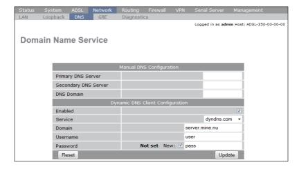
Finish and activate the settings by clicking on *Update*, the DDNS client will now track the changes of the ADSL interface of the ADSL-350 and update the domain server.mine.nu should the unit get a new IP address.
