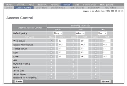
In this view some of the most common services are listed and their current firewall status. In our example we wanted the unit to respond to incoming requests destined to the web-interface on the ADSL interface IP (DSL-1). Just tick the **Allow** tickbox and then click on **Update**. The settings are activated immediately and the ADSL-350 can now be accessed from the Internet.
