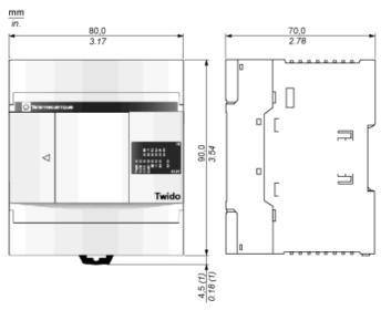
(1) 8.5 mm (0.33 in) when the clamp is pulled out.
