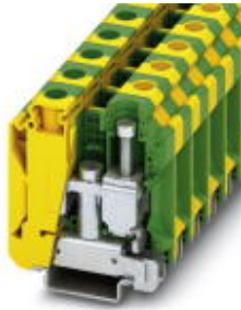
Ground modular terminal block, Connection method: Screw connection, Cross section: 10 mm 2 - 35 mm 2 , AWG: 8 - 2, Width: 16 mm, Color: green-yellow, Mounting type: NS 35/7,5, NS 35/15
