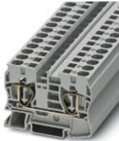
Feed-through terminal block, Connection method: Spring-cage connection, Cross section: 0.2 mm 2 - 16 mm 2 , AWG: 24 - 6, Width: 10.2 mm, Color: gray, Mounting type: NS 35/7,5, NS 35/15
