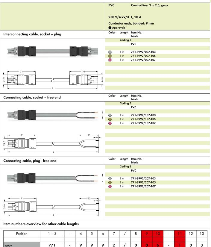
The item numbers listed above correspond to the following cable version: Interconnecting cable, 2-pole, socket - plug, PVC control line,  $2 \times 1.5 \text{ mm}^2$ , 1 m
