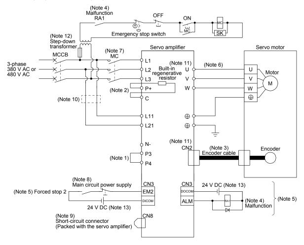
Note 1. Always connect between P3 and P4 terminals. (factory-wired) When using the power factor improving DC reactor, refer to section 9.8. Use either the power factor improving DC reactor or the power factor improving AC reactor.
