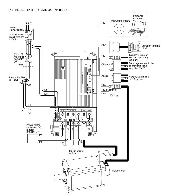
Note 1. The power factor improving AC reactor can also be used. In this case, the power factor improving DC reactor cannot be used. When not using the power factor improving DC reactor, short P3 and P4.
