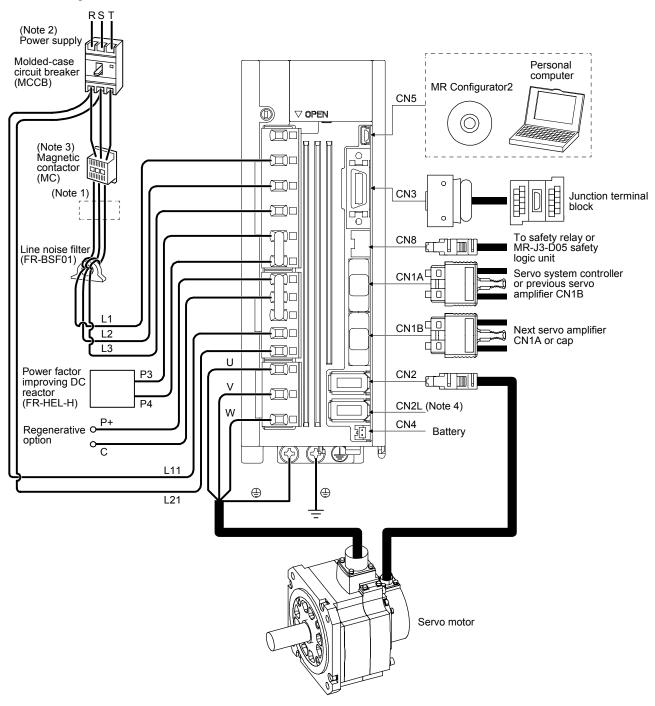
Note 1. The power factor improving AC reactor can also be used. In this case, the power factor improving DC reactor cannot be used. When not using the power factor improving DC reactor, short P3 and P4.
