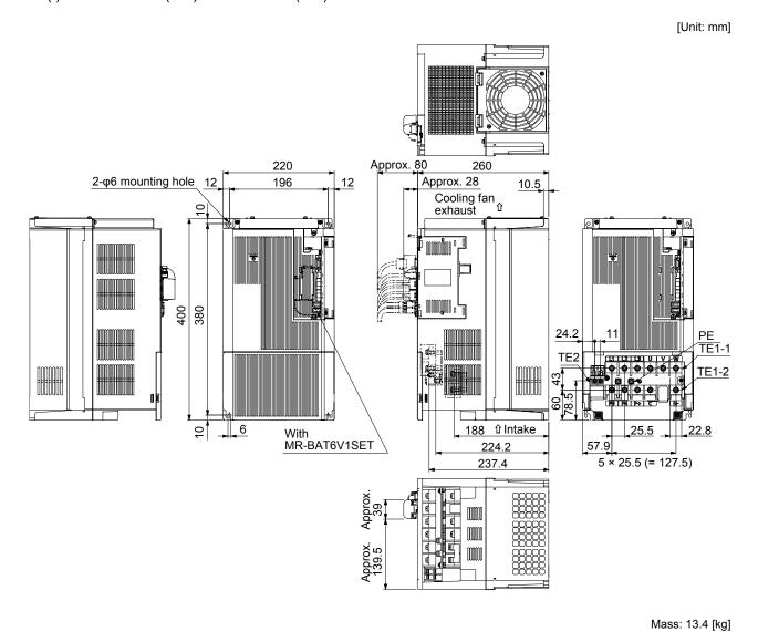
Terminal TE1-1 L1 L2 L3 U V W TE1-2 P3 P4 P+ C TE2 L11 L21 PΕ TE1-1 Screw size: M6 Tightening torque: 3.0 [N•m] TE1-2 Screw size: M6 Tightening torque: 3.0 [N•m] TE2 Screw size: M4 Tightening torque: 1.2 [N•m] PΕ Screw size: M6 Tightening torque: 3.0 [N•m]
