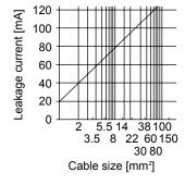
Fig. 9.7 Example of leakage current per km (lg1, lg2) for CV cable run in metal conduit
