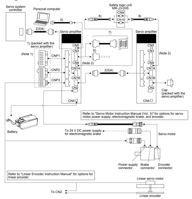
Note 1. Connectors for 3.5 kW or less. For 5 kW or more, it is a terminal block.
