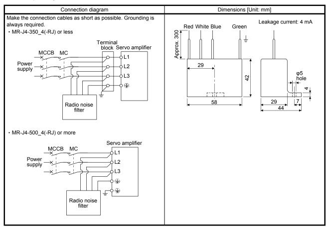
(f) Varistor for input power supply (recommended) Varistors are effective to prevent exogenous noise and lightning surge from entering the servo amplifier. When using a varistor, connect it between each phase of the input power supply of the equipment. For varistors, the TND20V-102K, manufactured by NIPPON CHEMI-CON, are recommended. For detailed specification and usage of the varistors, refer to the manufacturer catalog.
