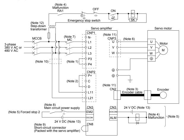
Note 1. Always connect between P3 and P4 terminals. (factory-wired) When using the power factor improving DC reactor, refer to section 9.8. Use either the power factor improving DC reactor or the power factor improving AC reactor.
