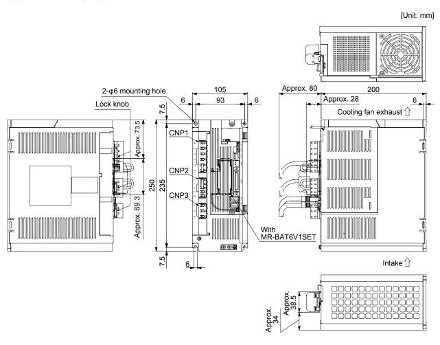
Terminal CNP1 N-L1 L2 L3 РЗ P4 CNP2 P+ С D L21 CNP3 U ٧ W Screw size: M4 Tightening torque: 1.2 [N•m] **(1)**  $\oplus$
