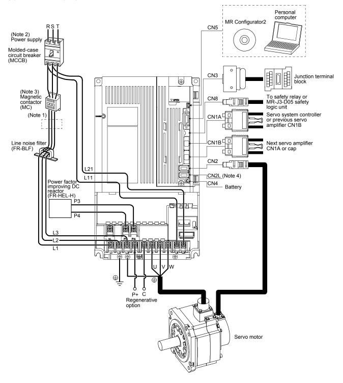
Note 1. The power factor improving AC reactor can also be used. In this case, the power factor improving DC reactor cannot be used. When not using the power factor improving DC reactor, short P3 and P4.
