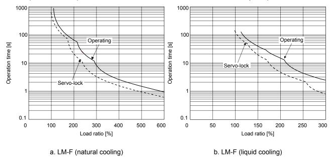
Fig. 10.1 Electronic thermal protection characteristics
