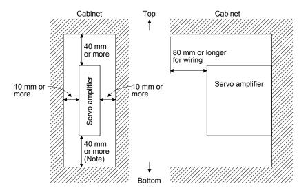
Note. For 11 kW to 22 kW servo amplifiers, the clearance between the bottom and ground will be 120 mm or more.
