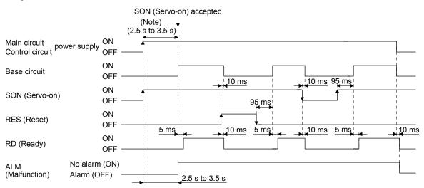
Note. This time period is longer when detecting magnetic pole for the linear servo motor.
