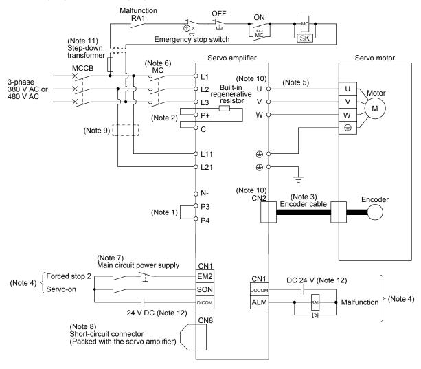
Note 1. Always connect between P3 and P4 terminals. (factory-wired) When using the power factor improving DC reactor, refer to section 9.8. Use either the power factor improving DC reactor or the power factor improving AC reactor.
