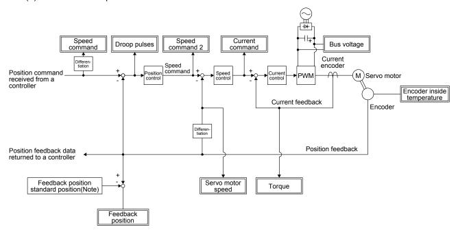
Note. The feedback position is output based on the position data passed between servo system controller and servo amplifier. [Pr. PC13] and [Pr. PC14] can set up the standard position of feedback position that is output to analog monitor in order to adjust the output range of feedback position. The setting range is between -9999 pulses and 9999 pulses.
