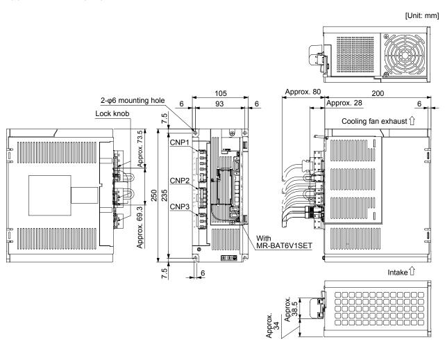
Terminal CNP1 N-L1 L2 L3 P3 P4 CNP2 С D L21 CNP3 U V W PE Screw size: M4 **(4)**  $\oplus$ Tightening torque: 1.2 [N•m]
