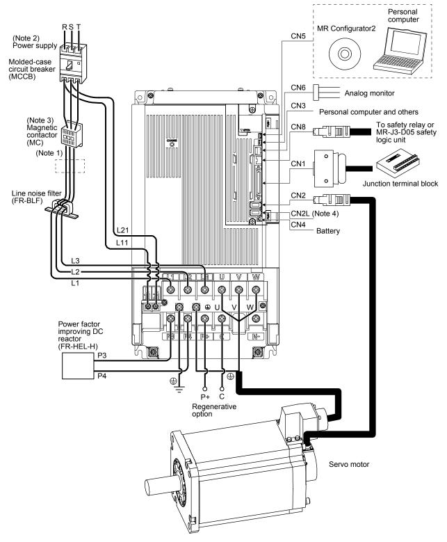
Note 1. The power factor improving AC reactor can also be used. In this case, the power factor improving DC reactor cannot be used. When not using the power factor improving DC reactor, short P3 and P4.
