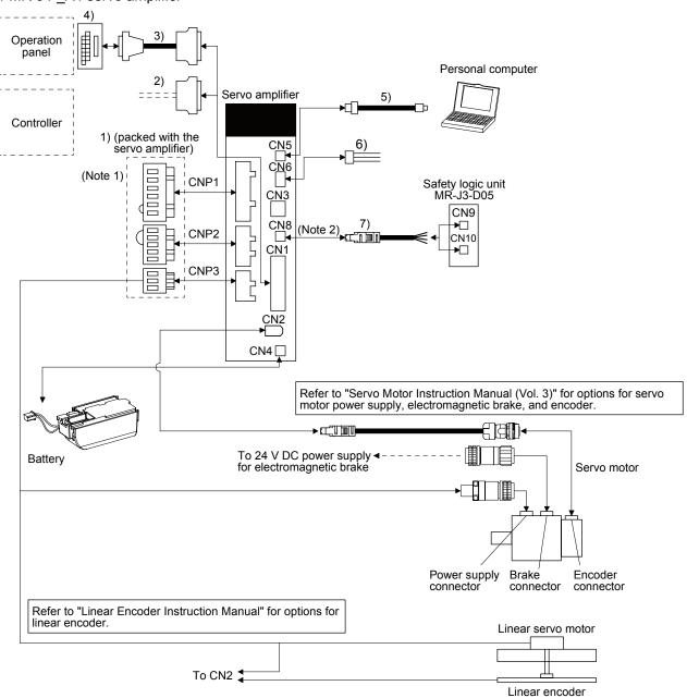
Note 1. Connectors for 3.5 kW or less. For 5 kW or more, it is a terminal block.
