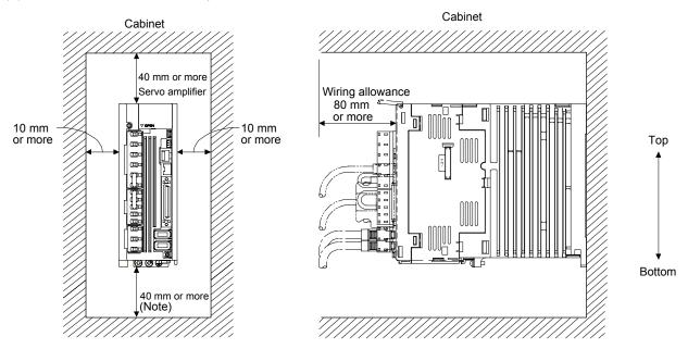
Note. For 11 kW to 22 kW servo amplifiers, the clearance between the bottom and ground will be 120 mm or more.
