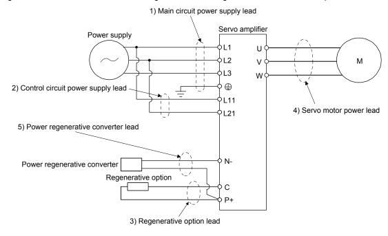
(1) When using the 600 V Grade heat-resistant polyvinyl chloride insulated wire (HIV wire) Wire size selection examples for HIV wires are indicated below.
