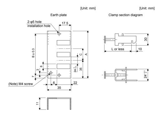
Note. Screw hole for grounding. Connect it to the grounding plate of the cabinet.
