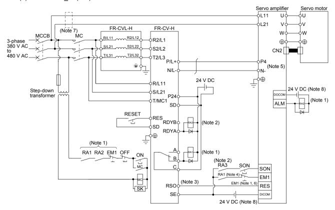
Note 1. Configure a sequence that will shut off main circuit power in the following.
