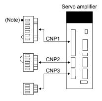
Note. A pin for preventing improper connection is inserted to N- of CNP1 connector.
