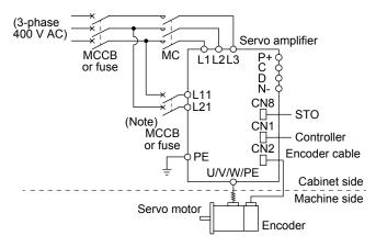
Note. When the wire sizes of L1 and L11 are the same, MCCB or fuse is not required.
