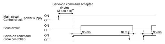
Note. This time period is longer when detecting magnetic pole for the linear servo motor.
