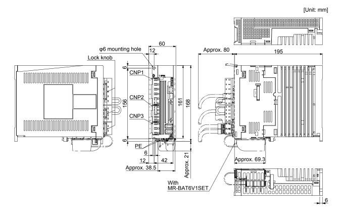
Terminal CNP1 N-L1 L2 L3 P3 P4 CNP2 P+ C D L11 L21 CNP3 U V W PΕ Screw size: M4  $\oplus$  $\oplus$ Tightening torque: 1.2 [N•m]
