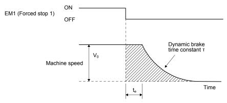
Fig. 8.3 Dynamic brake operation diagram
