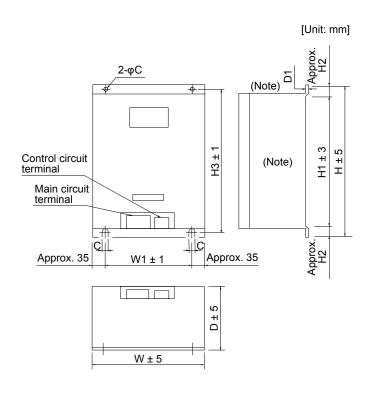
Note. Ventilation ports are provided on both sides and the top. The bottom is open.
