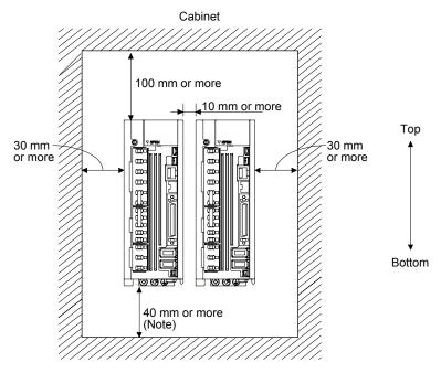
Note. For 11 kW to 22 kW servo amplifiers, the clearance between the bottom and ground will be 120 mm or more.
