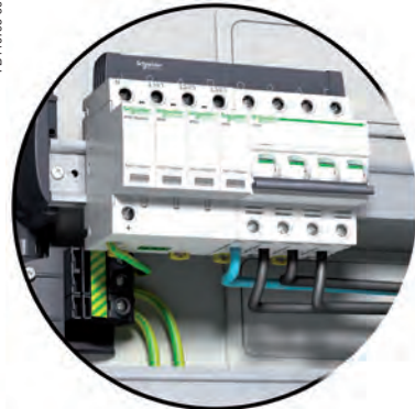
Surge arrester iPRD 3P+N + iC60 3P+N for TT or TN-S (Incoming through the bottom with comb busbar)
